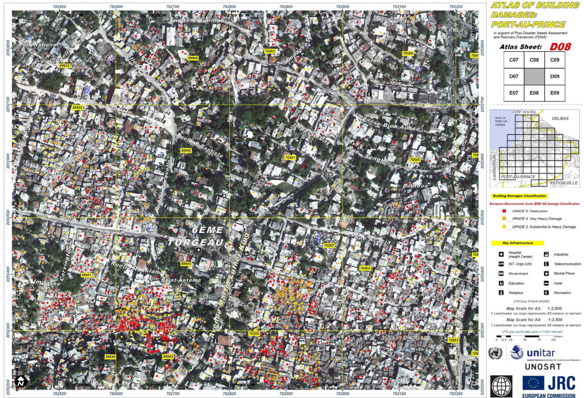
Figure 3: This map shows an example of an atlas map sheet with the aerial photograph in the background, the identified damages and additional information such as road names.
